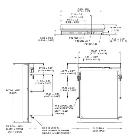
Figure 3. Mounting dimensions—top, side and end view
