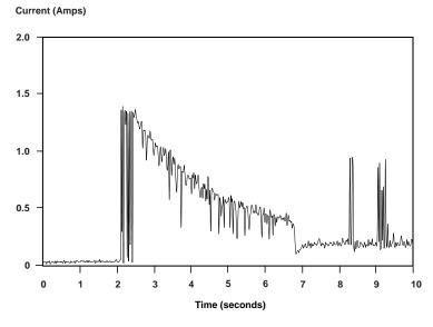
Figure 1. Typical startup and operation current profile
