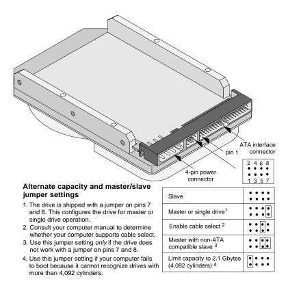
Figure 2. Alternate capacity jumper and master/slave jumper
